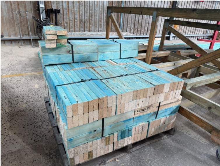
Figure 14: Blocks cut out of reject boards from MGP 10 packs
