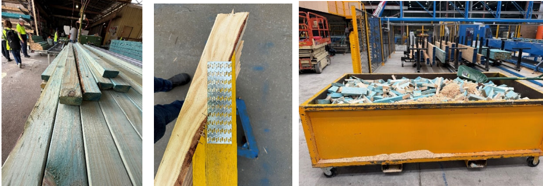
Figure 15: Timber grade characteristics that can cause problems during F&T manufacturing. Knots and resin pockets (Top Left). Spring (Top Middle). Resin pocket (Top Right). Wane (Bottom Left and Bottom Middle). Wasted offcuts (Bottom Right).
